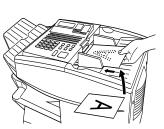
Note: When inserting a large number of pages in the feeder, slant the front end of the stack so that the bottom pages enter first.
